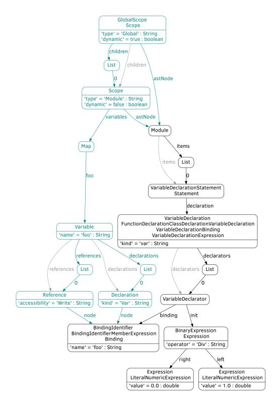
Figure 2.4 AST (in black) with additional edges (ASG, in turquoise) and derived helper edges (in gray).
