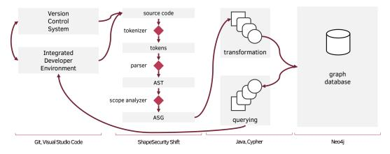
Figure 4.1 Architecture overview of the approach.
